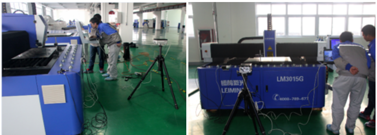
Use international high-end laser interferometer to detect machine dynamic performance
